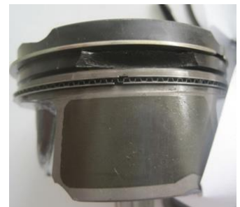
Piston ring land crack
